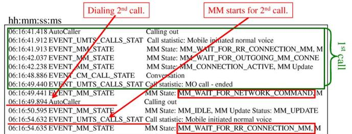
Fig. 6. A signaling trace of a delayed-call example. The dialing is delayed for about 5 seconds by MM.
