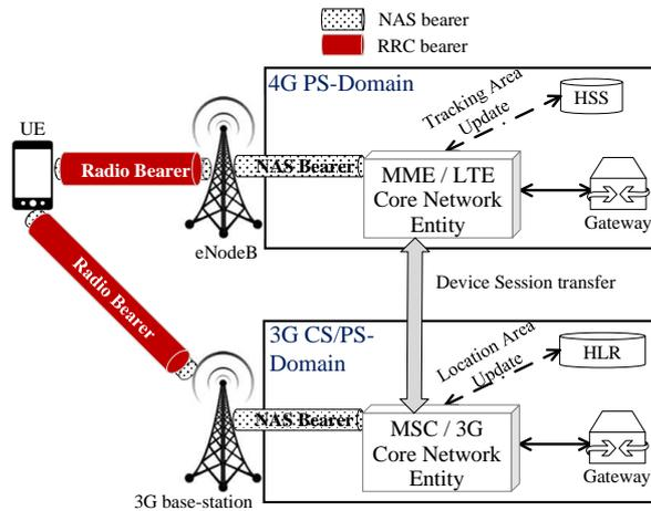
Fig. 2. Inter-radio access technologies (IRAT) interaction
