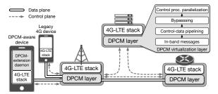
Figure 6: DPCM's system components.
