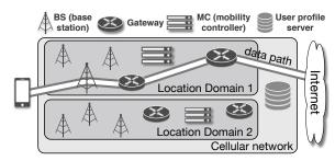
Figure 1: LTE network architecture.
