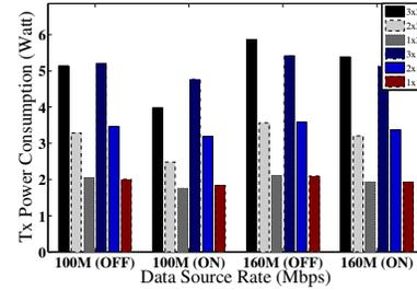
(b) Transmitter power consumption (Watt).
