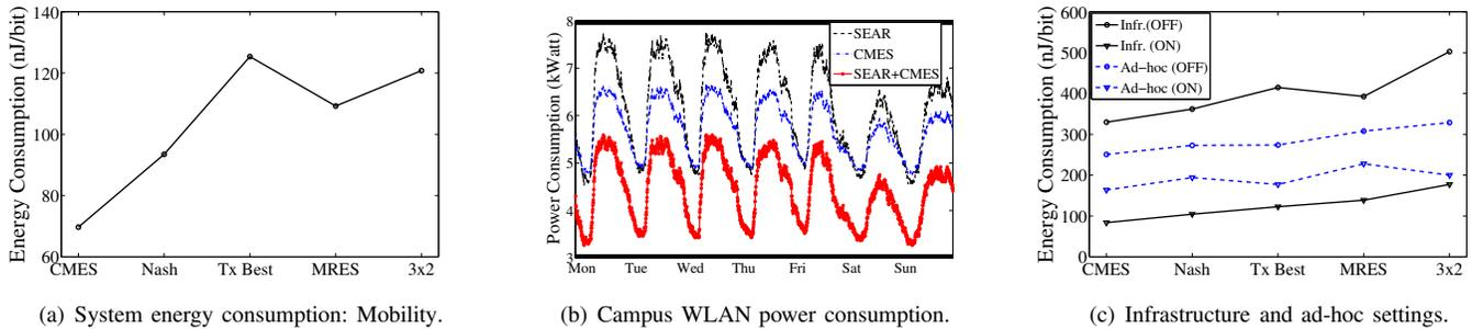
Fig. 12. System per-bit energy consumption (nJ/bit) for mobility and larger network topologies.
